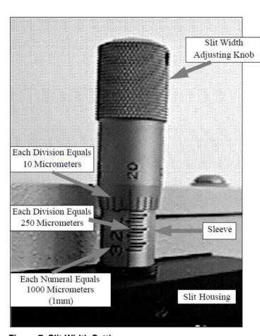
Figure 7. Slit Width Setting: 200 Micrometers (0.200 mm)
